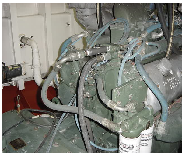
ECO-5 installed on both 12V 149 Detroit Engines
