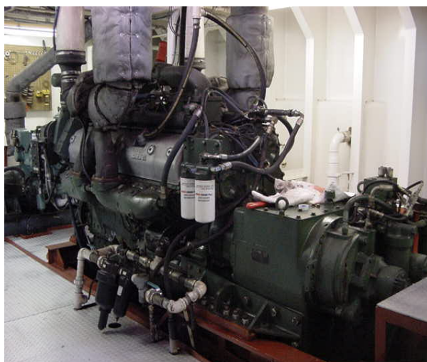
ECO-5 installed on both 12V 149 Detroit Engines
