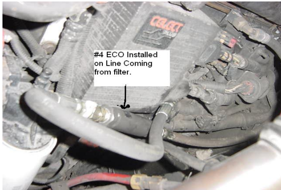
ECO-4 Installed on Cummins Engine
